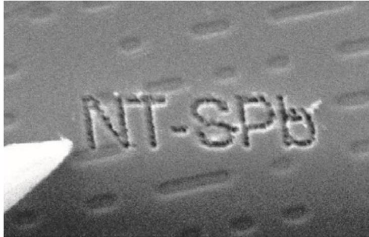
Figure 2. SEM image of a result of a dynamic force nanolithography performed under electron beam control in SPM combined with SEM. (on the left the W-probe used for probe nanolithography is seen, scanning area  $6 \times 7 \mu\text{m}^2$ ).
