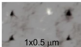
Figure 2. Indentation imprints of the treated surface.
