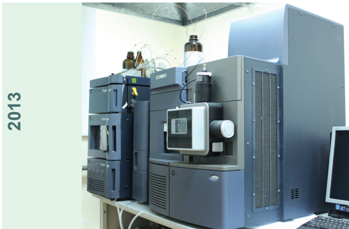
Quadrupole (Q) and time-of-flight (ToF) high resolution mass spectrometer
