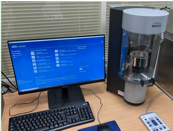
Tensiometer with a module for measuring the critical concentration of micelle formation
